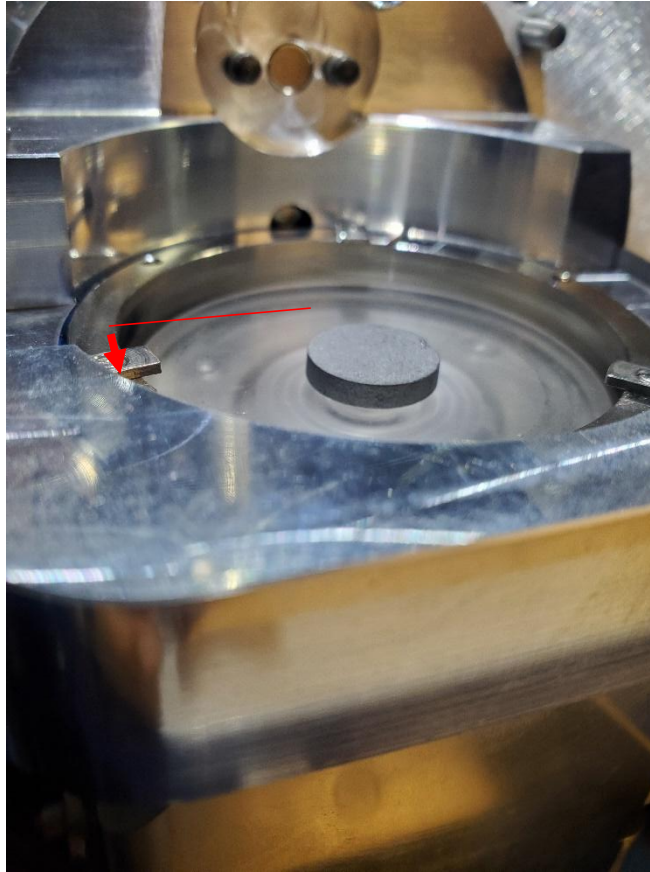
Figure 5. Sample height is going below the level in the machine during measurement. The required level is shown by a line while the unreached height is shown by the arrow. This position is wrong for the stage during measurement.
