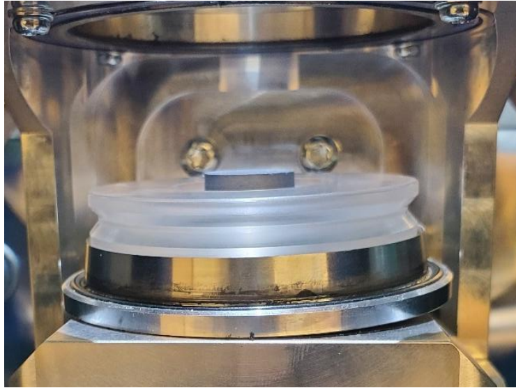
Figure 3. Sample Pellet thicker than the sample holder depth where sample goes.
