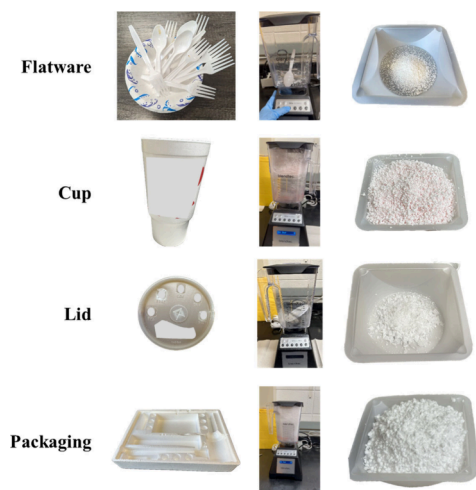
Figure 1. Samples of postconsumer polystyrene used for this study showing the items as-collected (left column), during grinding (middle column), and after grinding (right column). Grey shapes have been added to the as-collected images of the cup and lid to cover trademarked images of the restaurant chain from which the refuse samples were collected.
