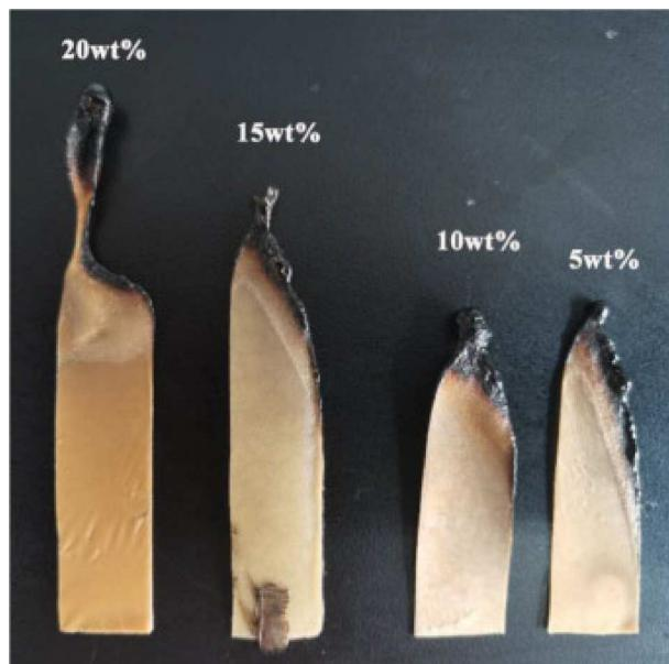
**Figure 24.** A photograph depicting the residual state of burned composite materials. Reprinted with permission from the published source (20). Copyright 2022 Elsevier.
