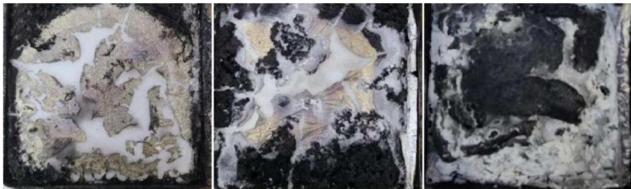
**Figure 32.** Char after the Cone Calorimeter Test for (a) EP, (b) EP/8CNC@DPP, and (c) EP/8CNC@DPP@Zn. Reprinted with permission from the published source (86). Copyright 2022 John Wiley and Sons.
