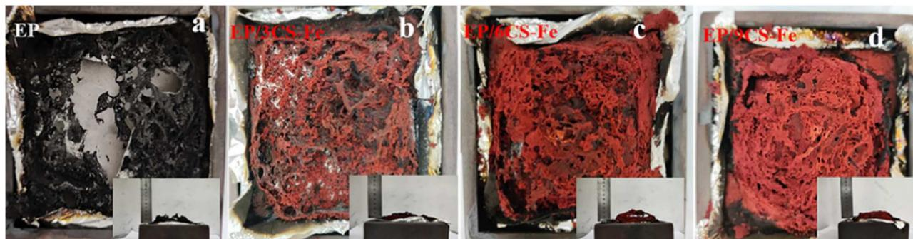
**Figure 30.** (a) EP char, (b, c, d) EP/CS-Fe composites after CC test. Reprinted with permission from the published source (85). Copyright 2022 American Chemical Society.
