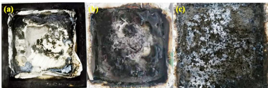
**Figure 26.** The digital photos of the burning residues after CCT analysis. Reprinted with permission from the published source (83). Copyright 2022 Springer Nature.
