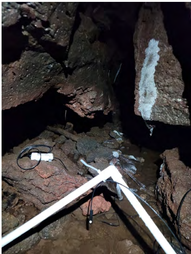
Figure 3. Ice puddle monitoring in Bonito Flow Ice Cave (location 4 on figure 2 and table 1 ). A PVC pipe constructed tripod was used to hang a sensor probe above the ice puddle to monitor air temperature/humidity. Additional temperature/humidity sensors were located at this site to measure the ice and rock surface temperature and humidity. Photograph taken by Timothy Titus, U.S. Geological Survey.
