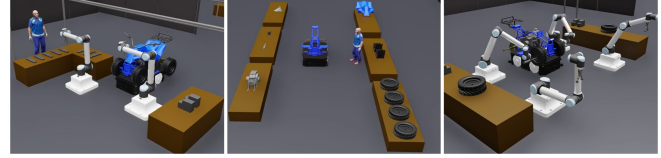
Fig. 1: An example of a human multi-robot assembly cell for producing all-terrain vehicles in high-mix low-volume has been developed in simulation. When coordinating all agents, task scheduling methods must take into account human preferences, as well as dynamic changes in task requirements and the environment.
