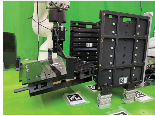
Fig. 2. An example of a contingency occurring during the assembly process. The robot fails to insert the battery sub-assembly into the main assembly, requiring additional contingency tasks to be executed.
