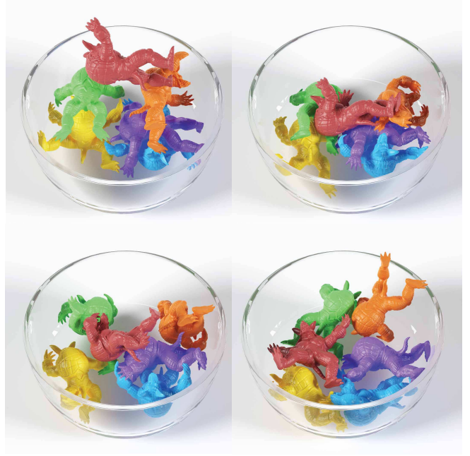
Fig. 4. Falling Armadillos. Six Armadillo models consist of 1.2M vertices and 6M elements. They collide with each other while falling into a container. Our method requires an average of 58 iterations per time step with h = 1/150 , compared to 44 iterations for the projected Newton method. However, our method requires only 883 ms per step, achieving a speedup of approximately 8000× compared to the projected Newton method, which takes 106 minutes per step.
