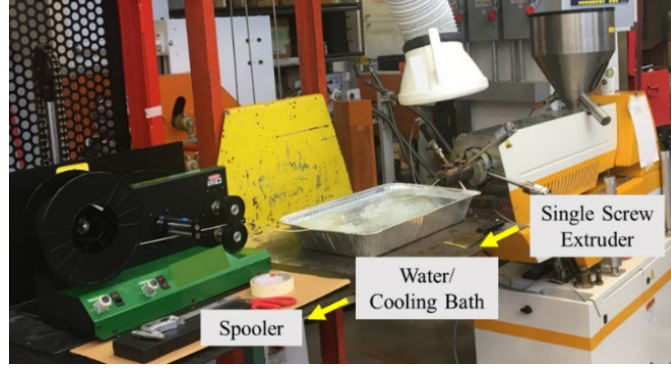
Figure 1. Single-screw extrusion setup with cooling bath and filament spooler used for the fabrication of unexpanded filaments.
