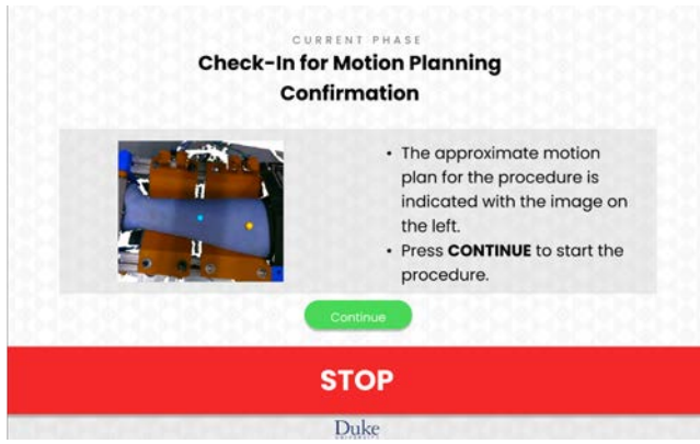
Fig. 2: Check-in step for User Interface for Participant to approve approximate motion plan
