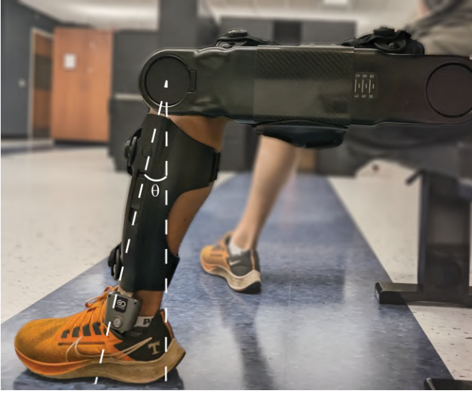
Figure 1. Exoskeleton testbed used to simulate tremor and to measure the knee joint angle ( \theta in the image).
