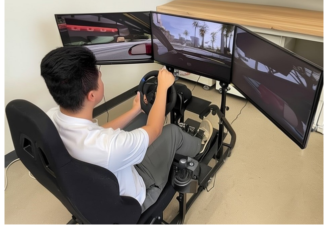
Fig. 5. The driver-in-the-loop simulator with CARLA used by Driver 1 & Driver 2.
