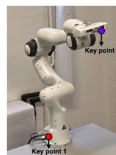
FIGURE 5. Pose detection example from the RoboMNIST dataset showing two key points annotated on the robotic arm: Key Point 1 (base of the arm, highlighted in red) and Key Point 2 (end effector, highlighted in purple).
