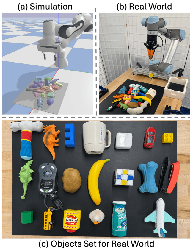
Fig. 6. Experiment Setup. The workspace is a 40\text{ cm}^3 cube in both environments. The training and test object sets in simulation follow [14], while the real-world object set is shown in (c).
