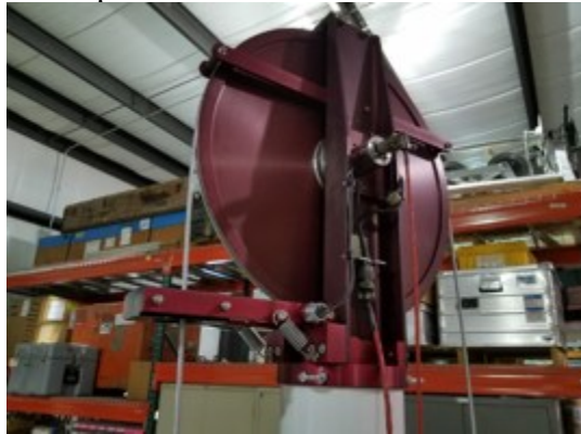
Figure 9: Foro 400 crown sheave with spring-loaded cable guide.
