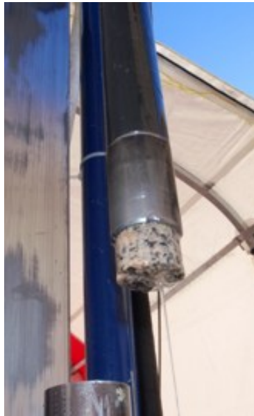
Figure 38: The first subglacial rock core drilled using the ASIG Drill system. Core breaks are performed using a collet inside of the drill head.
