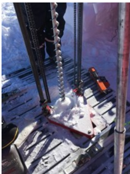
Figure 41: At the Ohio Range, access holes were drilled in ice using Kovacs 2-inch augers.
