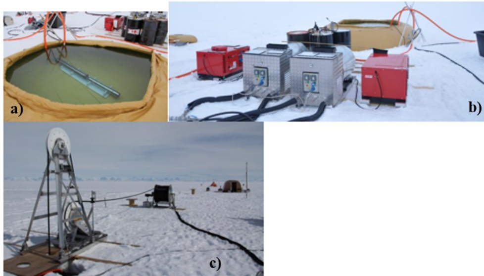
Figure 51: Ice shelf HWD, 500 m configuration. a) Primary drill pump 5.5 kW submersible pump in water tank, b) 250 kW water heaters without heat recovery units and 15 kVA generator (red) with one on standby, and c) the hose winch reel, capstan, and tower with instrumented sheave.
