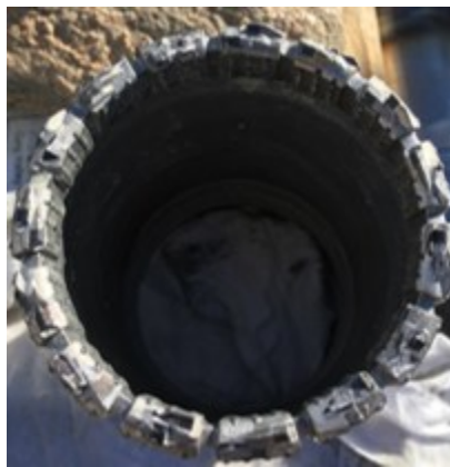
Figure 44: This Geoset style coring bit was used exclusively in Ong Valley where only mixed media was cored.
