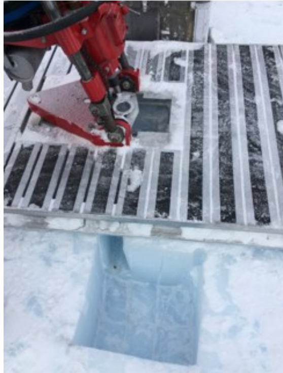
Figure 45: Sump pit cut from the solid blue ice at the surface. The drill fluid is pumped through the drill rod and returns to the surface where it is collected in the sump.
