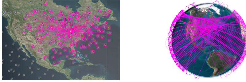
Figure 2: Locations of 650 simulated Starlink SVs over Columbus Ohio, USA (left) and their corresponding 3-D trajectories (right).
