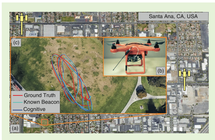
FIGURE 4. The 5G experimental results: the (a) environment layout, (b) UAV, and (c) UAV trajectory: ground truth and estimated with the known beacon versus COSON.
