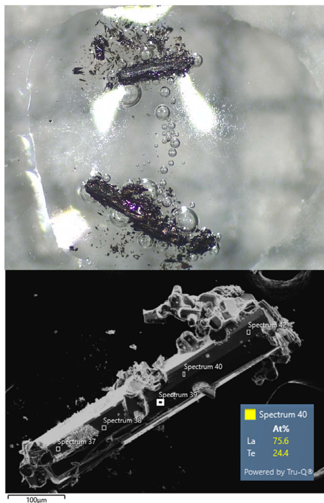
Figure 1. Top: Microscope image on mm grid paper of crystals of \text{La}_3\text{BiC}_2 reacting in a drop of water. Bottom: Scanning electron microscope image of a crystal of \text{La}_3\text{TeC}_2 , along with SEM-EDS elemental analysis.
