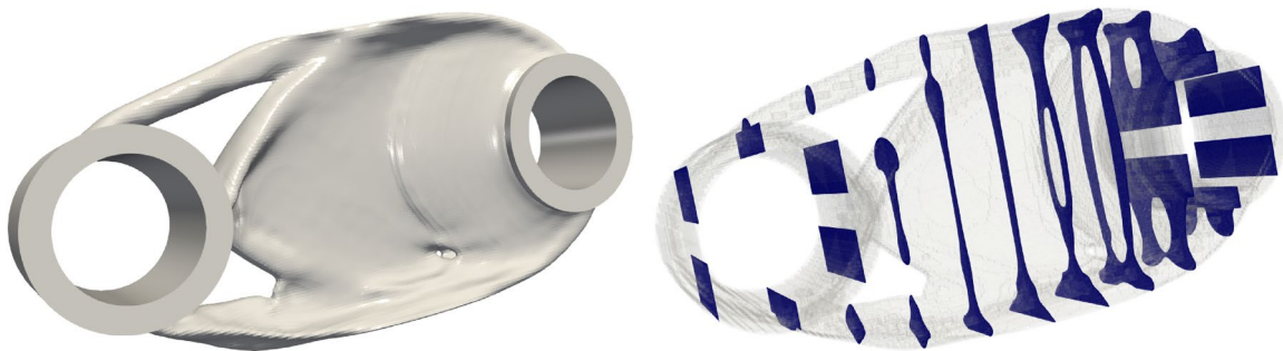
Fig. 16 Three-dimensional optimization result (left); final design and cross-sections (left)
