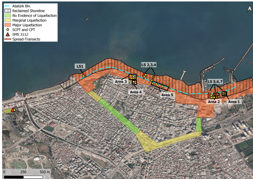
Figure 6. Overview of liquefaction observations and demarcation of key study areas within İskenderun.
