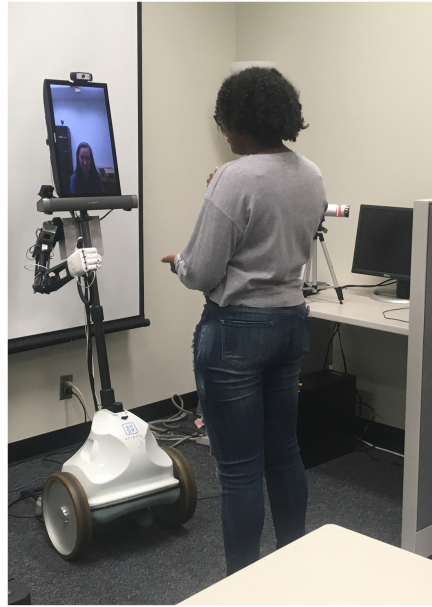
Fig. 6. The experimental setup of the local user experiments illustrating a subject interacting with the telerobot with the arm attached. The same set-up was used for the no-arm condition with the same robot, but the arm was removed.
