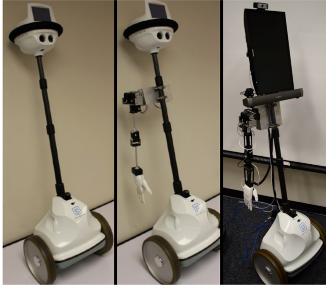
Fig. 1. The Anybots QB 2.0 (left), the platform modified with the initial manipulator (center) [41], and the current modified platform (right).
