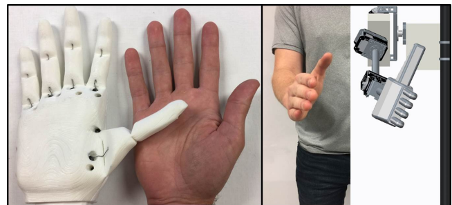
Fig. 2. Left: The hand, an Open Bionics Ada Hand, used in the manipulator design compared with a human hand. Right: The 4 DOF manipulator replicating normal handshake tilt.
