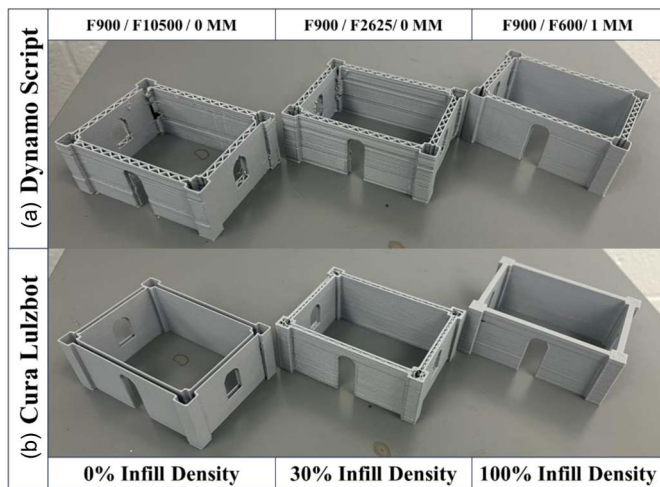
Fig. 15. Printing samples and quality evolution to adjust printing settings.
