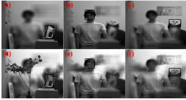
FIGURE 5. (a)–(c) 3D integral imaging reconstruction of the clear scene shown in Fig. 2(a) at each of the object's depths - the iron, the mannequin, and the thermal mannequin respectively. (d)–(f) 3D integral imaging reconstruction of the partially occluded scene shown in Fig. 2(b) at each of the object's depths - the iron, the mannequin, and the thermal mannequin respectively. In each 3D reconstruction, the object in focus is circumscribed with a black colored box.
