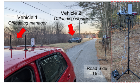
Fig. 8. Road tests experimental setup.
