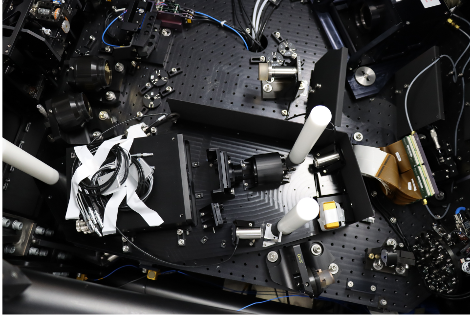
Figure 5: The WFS immediately after being installed on the OMSS optical bench. The tall white poles were used for alignment
