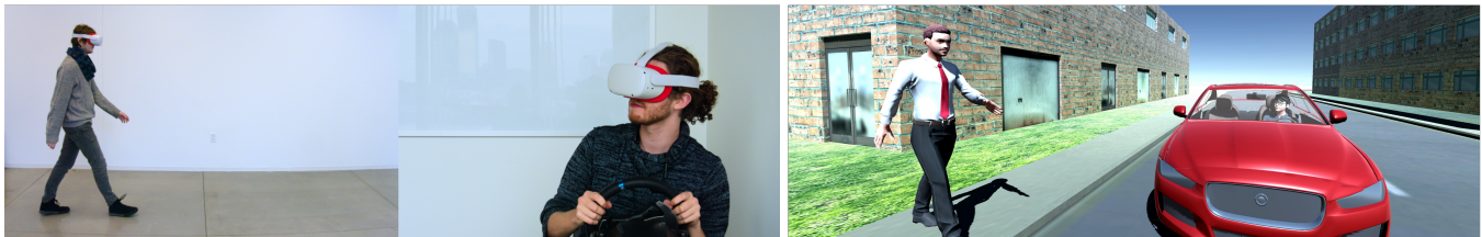
Figure 1: GrokWalks is a portable, multi-participant simulator platform that facilitates studying naturalistic driver-pedestrian interaction in a virtual environment: the images above show real-life and virtual representation of interacting participants.
