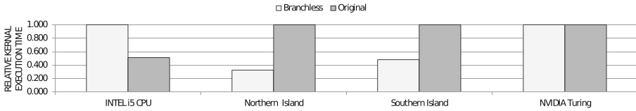
Fig. 1. Relative execution time for experiment code. Branched version is compared to the flattened, branch-less version on four different processors. The processors and compiler scenarios are described in Sect. 4.
