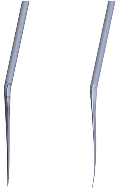
Fig. 2 Modeled geometry of GRB's straight (left) and curved (right) blade paddles in a side by side configuration.
