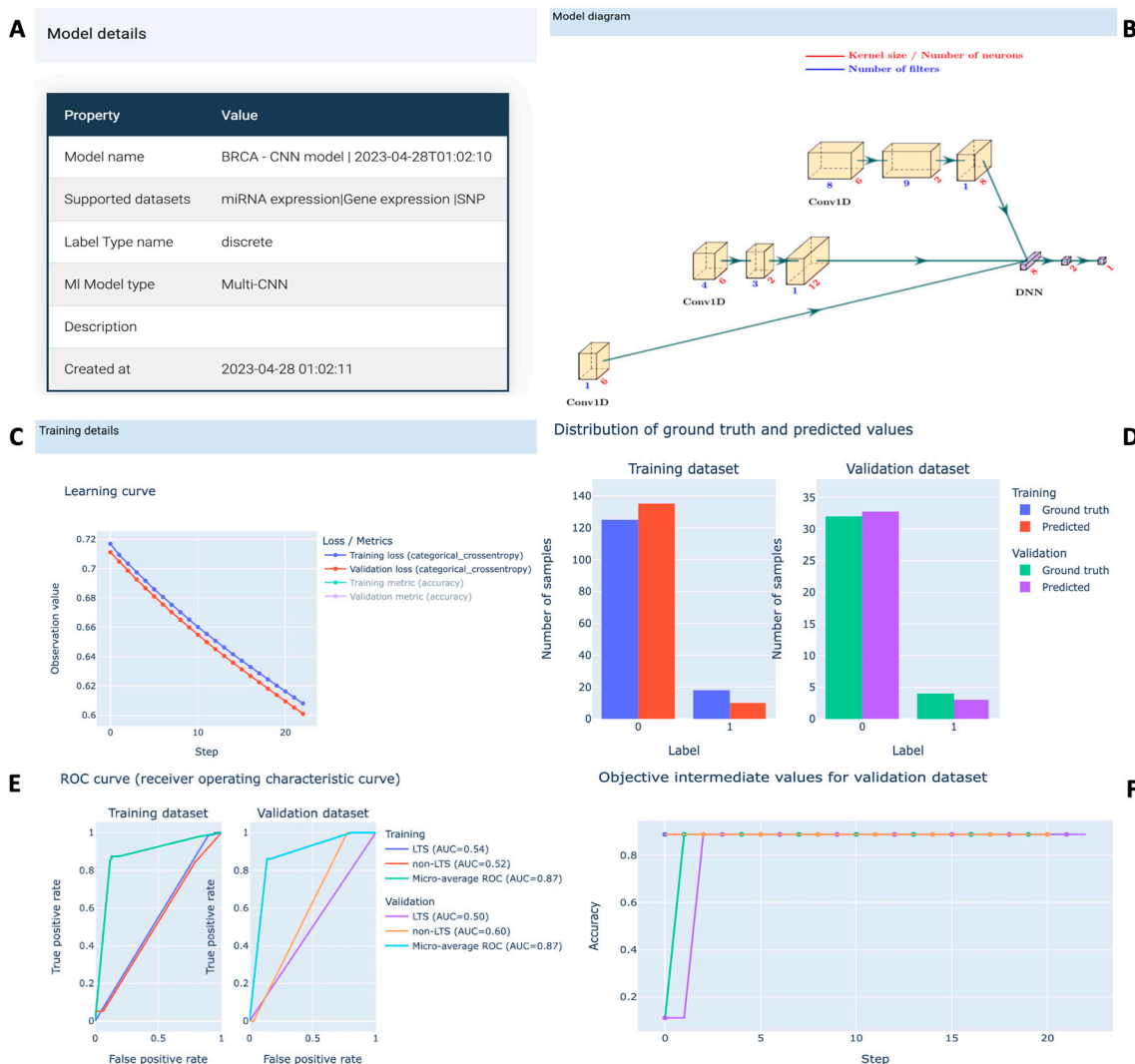
Figure 6. Project page in G2PDeep-v2. (A) Model summary showing the type of model and corresponding training dataset; (B) visualization of the multi-CNN architecture, illustrating the convolutional and fully connected layers used for multi-omics feature extraction and integration; (C) learning curves showing training and validation loss across epochs, allowing users to monitor model convergence and potential overfitting; (D) distribution of ground and predicted values for training and validation datasets; (E) ROC for phenotype prediction, demonstrating the discriminative ability of model on training and validation datasets; (F) optimization history from the Bayesian hyperparameter tuning process, highlighting how model performance improves over successive iterations of parameter adjustment. Each line represents a single trial.
