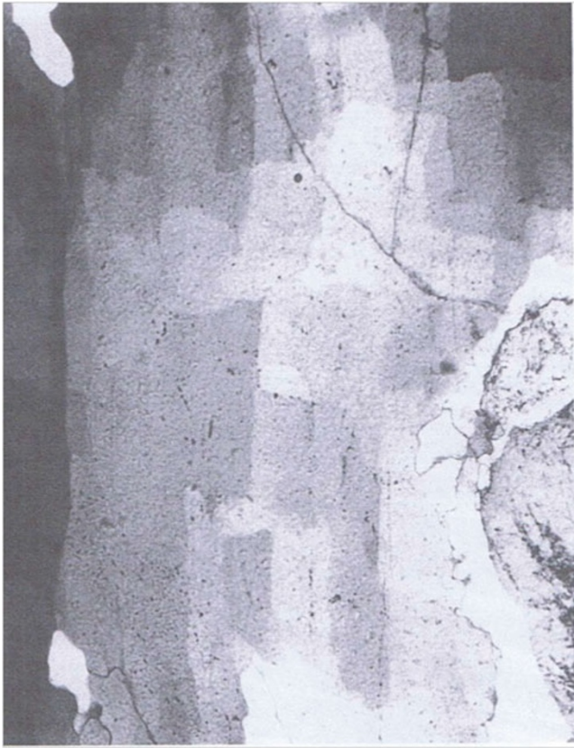
Figure 2. Chessboard-patterned subgrain domain development in high-temperature metamorphosed quartz, Great Zimbabwe, Zimbabwe. Vertical domain boundaries are on prismatic planes, horizontal domain boundaries lie on basal planes. Horizontal dimension of the photomicrograph is \sim 1 mm. (BLENKINSOP, 2000, figure. 4.10; reprinted with the permission of Kluwer Academic Publishers).
