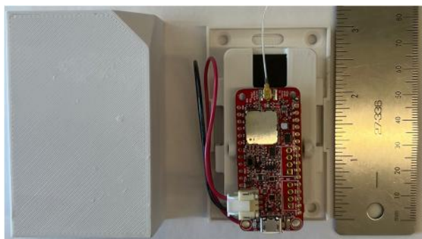
Fig. 3 MCCI Catena 4618 M201 IoT sensor within enclosure base, right. Enclosure cover, left. Seventy-three IoT sensors were distributed throughout the building in all rooms of each apartment unit and building common spaces to capture local thermal environment changes over the entire duration of the study.
