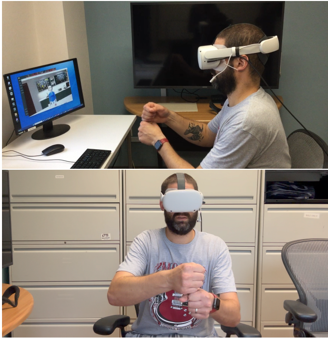
Figure 1: ASL Champ user experience set up. A user is signing coffee signs displayed on the VR headset mirrored on the computer monitor. The side and front views are shown on the left and right, respectively.
