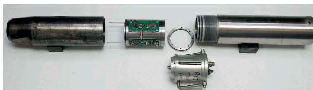
Figure F24. APCT-3 tool for in situ temperature measurements.
