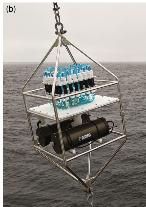
Fig. 1. (a) Schematic of MoRIS design from McLane Research Laboratories, Inc., and (b) photo of MoRIS during deployment in 2021.
