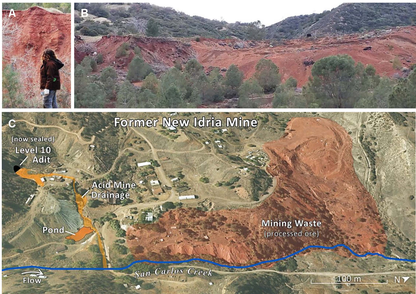
Fig 4. (A) Vertical wall of exposed mining waste along the channel of San Carlos Creek. (B) Profile view of waste piles with riparian vegetation in the foreground. (C) Oblique view of the former New Idria Mine showing AMD exiting the Level 10 Adit prior to EPA's remedial actions and the approximate extent of the solid waste piles.
