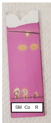
Figure 5: A) The reaction progress at 18hrs in KMnO 4 stain. To TLC 2, a drop of the reaction solution was removed and diluted with 0.5 mL of DCM. SM = 1.
