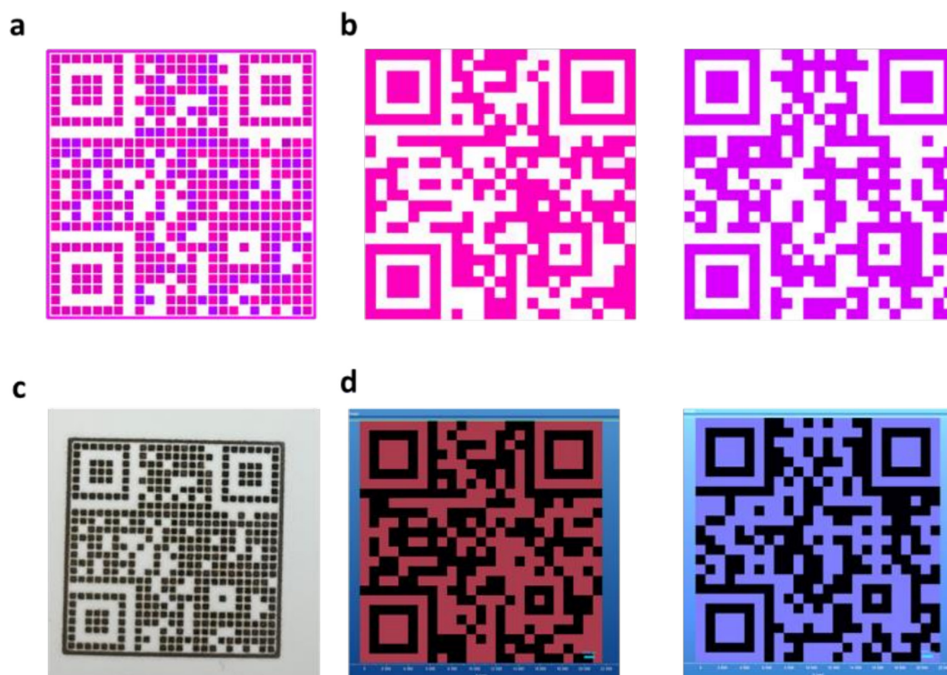
FIGURE 4 | (a) Pixelated dual QR code design; (b) left: QR code with RGB color code (255, 0, 191); right: QR code with RGB color code (217, 0, 255); (c) optical image of the dual QR code; (d) SERS mapping of the two different QR codes.
