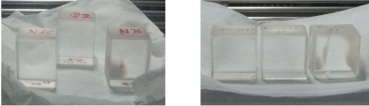
Figure 11: Left: A translucent layer is formed on WP with Norland 73 cement at lower temperatures ( = < -5^{\circ}\text{C} ). Right: Fracture developed in the WP with Norland 73 cement from the second set at -5^{\circ}\text{C} .
