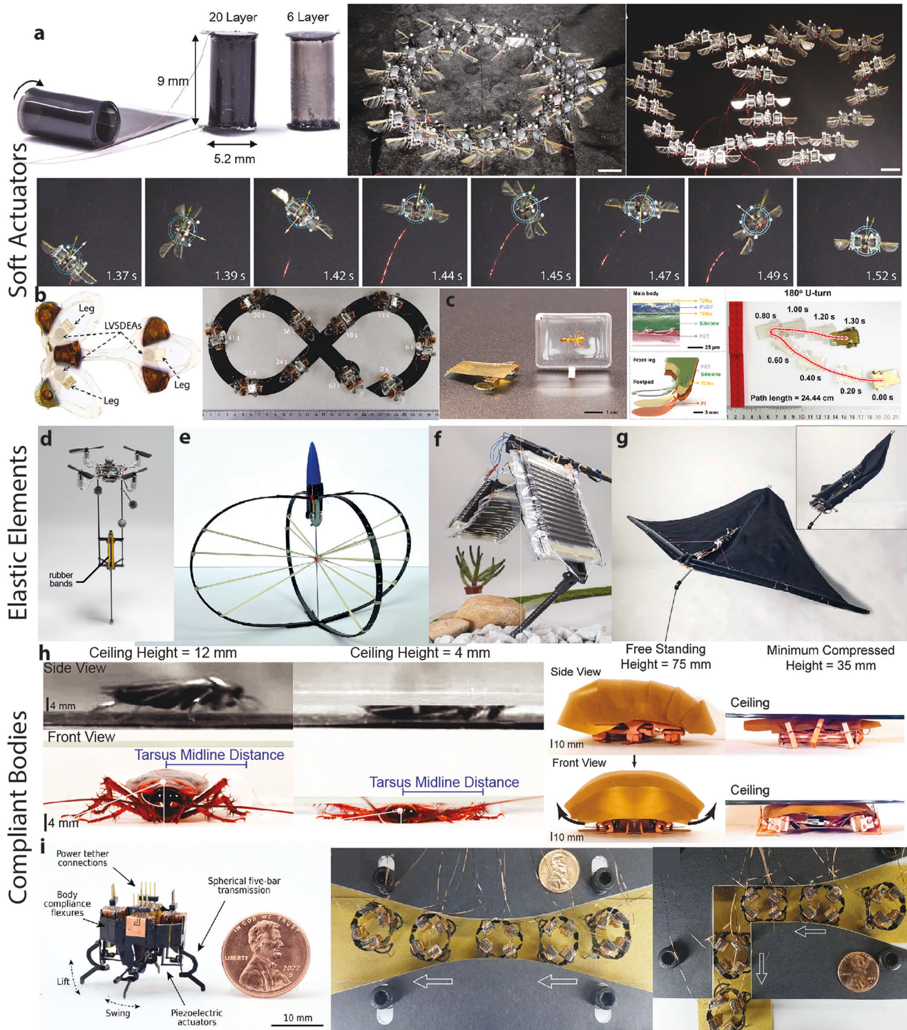
Fig. 2 | High-performance soft robots. Examples of systems that leverage muscle-like fast actuators, tendon-like energy storage mechanisms and flexible bodies for animal-like agility. a Driven by DEAs, miniature flying robots 46,50 are capable of high agility maneuvers, such as figure-8 motion or barrel rolls midflight. Similarly, b low-voltage stacked DEAs 64 and c PVDF-powered 160,161 legged robots demonstrate rapid planar locomotion. d–g Elastic elements of various forms enable high efficiency hopping 56,74 , record-breaking jump height 88 and deployable gliding via compliant
