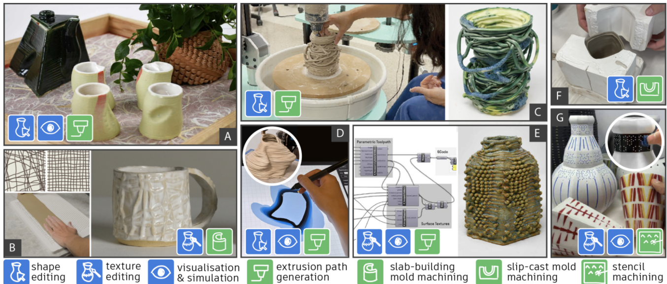
Figure 2: Computational Ceramics. Our course will introduce various opportunities in ceramic craft to leverage computational tools such as computer-aided design methods (blue icons) and computational fabrication techniques (green icons). We will use as examples the work of the course presenters. A: Bourgault et al. 2023 [Bourgault et al. 2023]; B: Bourgault et al. 2024 [Bourgault and Jacobs 2024]; C: Moyer et al. 2024 [Moyer et al. 2024]; D: Frost et al. 2024 [Frost et al. 2024]; E: Toka et al. 2023 [Toka et al. 2024]; F: work in progress; G: Toka et al. 2023 [Toka et al. 2023].
