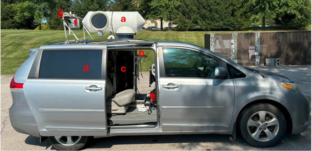
Figure S1. The COTS storm-intercept research vehicle (2013 Toyota Sienna). Light enters the optical pathway through a (a) 30.5-cm window in the periscope, where it is directed down into the vehicle by two \frac{1}{4} -wave flat turning mirrors. A small pickoff mirror directs some of this light to (b) the OFiL camera, a wider field-of-view, less sensitive version of the COTS UV camera, while the rest enters (c) a 25-cm diameter f4.0 Newtonian telescope, where it is focused into (d) the COTS visible and UV cameras. The system is powered by a battery and data are stored on either a digital video recorder or (e) a laptop hard drive. (f) The electric field mill measures the uncalibrated electric field
