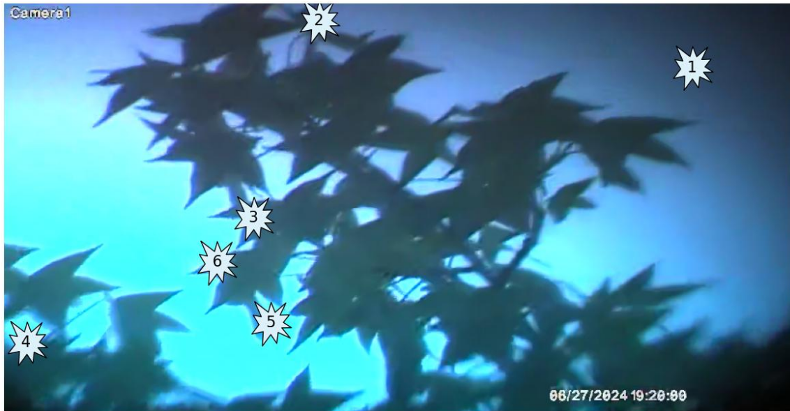
Figure S9. Six corona discharge UV signals observed during a 2.76 second period from 19:19:59 to 19:20:01 UTC on a sweetgum tree in Pembroke, NC on 27 June 2024. UV signals detected by the COTS UV camera are expanded, numbered by order of occurrence, and overlaid on the COTS visible camera closest to the location on the leaves where the signal occurred considering the leaves were moved across the frame by the wind (See Movie S1).
