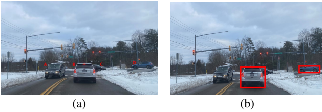
Fig. 2: (a) Image of a vehicle's front camera in which other vehicles block the view. (b) Objects detected by SSD.
